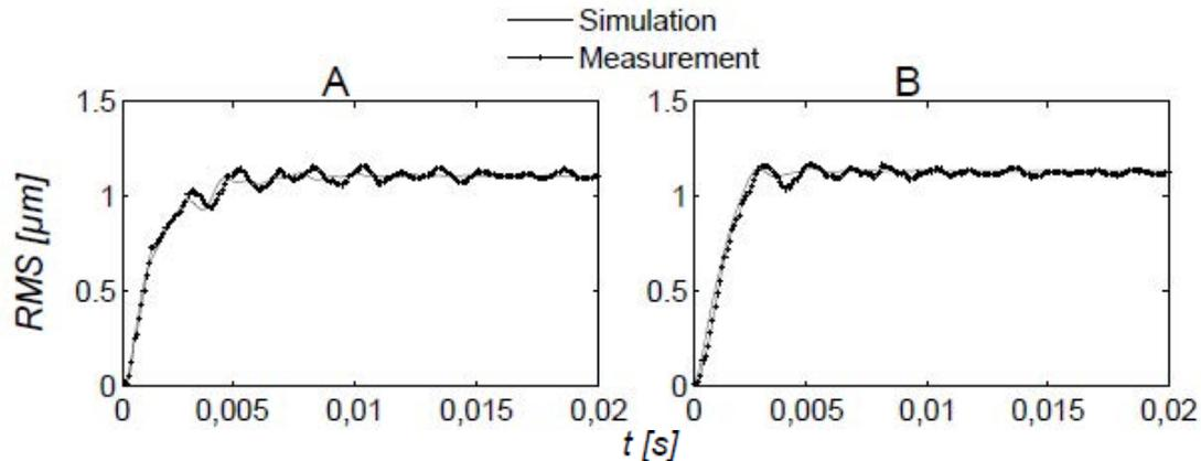
Fig. 1. Simulation and measurement of the DM's step response for a peripheral actuator when controlling the DM dynamic behavior by continuous- (A) and discrete- (B) time LQ control, respectively.
